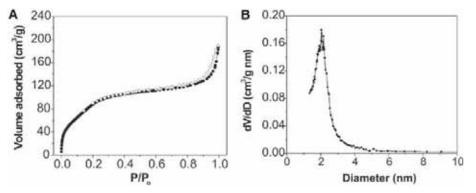
**Fig. 3.** (**A**) Nitrogen adsorption-desorption isotherms at 77 K of heat-treated  $NH_4^+$ -exchanged MSU-Ge-2 (solid circles, adsorption data; open circles, desorption data). The hysteresis observed at  $P/P_o > 0.8$  is due to the interparticle voids between the agglomerated particles. (**B**) BJH pore size distribution calculated from the adsorption branch of the isotherm.
